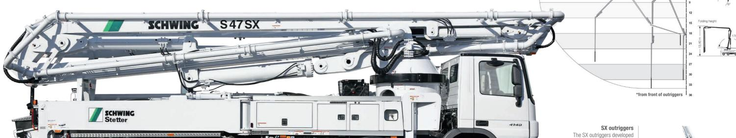
by SCHWING combine high torsional rigidity and excellent stability with minimum space requirement. The protected piston rod and internally laid hydraulic lines prevent damage and reduce service costs.
