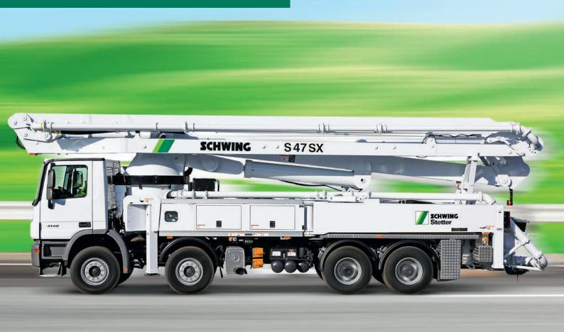
Vertical reach 46.40 m Concrete output max. 162 m³/h Pressure on concrete max. 85 bar
